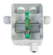
extinguishers. The ETB (Extinguishers Terminal Board) is equipped with built-in safety electronics to ensure all extinguisher igniters are activated. Together with an end of line switch, this option makes the system a complete and reliable fire detection and extinguishing release system. The ETB (Extinguishers Terminal Board) unit is available in a built-in 35 mm DIN rail version.
