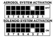
DS 3 OFF = system is suitable for electrical igniters intended for aerosol fire extinguishers 1,3A/50ms DS 3 ON = system is suitable for solenoid activation 24V DC 1 A
