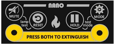
silence the external sounder, press the Mute button twice. In case of a second alarm the sounder and buzzer will be activated again.
