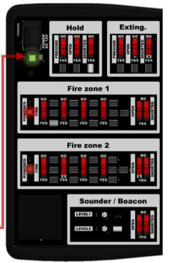
A fire alarm for each fire detector in each fire alarm zone can be simulated by setting the red switch into the YES position. A fire indication in 'fire alarm zone 1' on the NANO is the result. The red common FIRE
