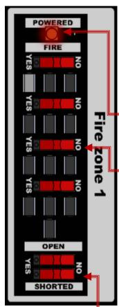
These resistors are also present on the FTM test module. All possible alarms and faults can be simulated by using the switches.
