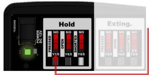
In the event of a fire alarm in both fire alarm zones or when operate the **EXTING** switch in the YES position, and an extinguishing release delay is programmed, the red 'delay' LED lite. When operating the **HOLD** switch, the tone signal will change, and the yellow 'hold' LED is lit in the 'Extinguishing' group. This
